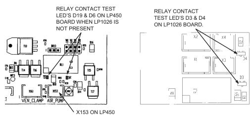
Figure 5 - Level Detector with Relay Contact Test LED's.
