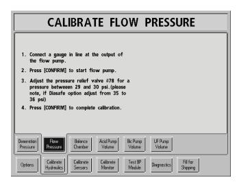
2. Connect a gauge in line at the **output** of the flow pump (See Figure 3, pg. 8).
