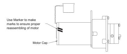
Figure 9. Deaeration Motor/Pump Assembly with marks.
