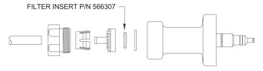
Figure 4. Concentrate and Bicarbonate Connector Assemblies.
