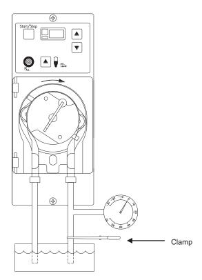
Figure 11. Blood Pump Rotor Occlusion Test
