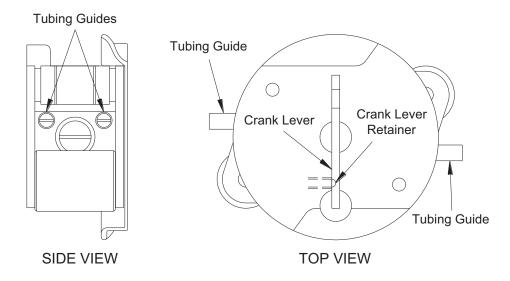
Figure 7. Blood Pump Rotor Assembly
