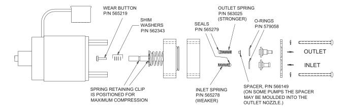
Figure 12. Ultrafiltration Pump Exploded View.
