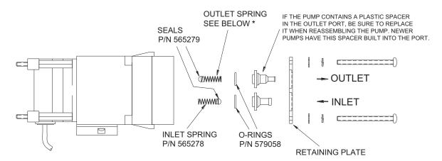
\* ON CONCENTRATE (ACID) PUMPS THIS SPRING IS STRONGER THAN THE INLET SPRING. USE P/N 563025. ON BICARBONATE PUMPS USE WEAK SPRINGS FOR BOTH INLET AND OUTLET (P/N 565278).
