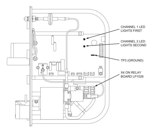
Figure 6 - Level Detector without Relay Contact Test LED's.
