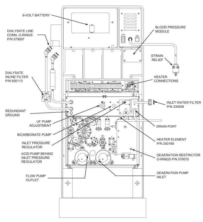
Figure 3. Fresenius 2008K Hemodialysis System, Rear View.
